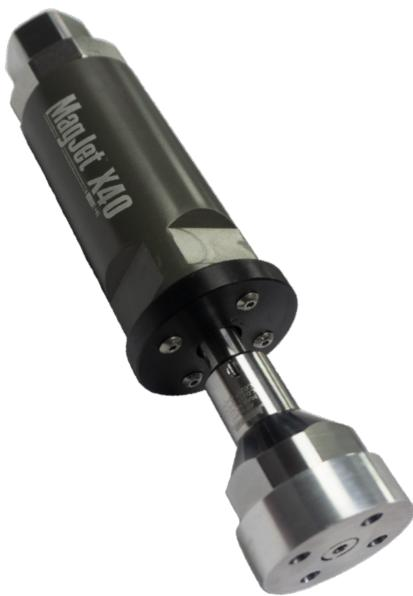
The Jetstream MagJet X40 is a rugged, self-powered, rotating tool utilizing up to four straight-pattern, hard-hitting, replaceable sapphire nozzles, rated up to 43,500 psi. The tool rotates in a 360° pattern to provide maximum surface coverage and superior cleaning.
