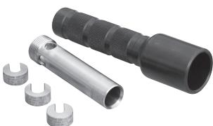
For use in flex lance tube cleaning operations, the safety grip prevents a nozzle from unexpectedly exiting a tube by providing a stop through which the sleeve of the flex lance will not pass. Package includes handle, lance stop retainer for use on tubes up to 3/4" O.D. Choose lance stop below (not included).
