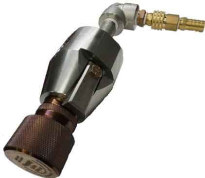
A bypass valve diverts a portion of pump flow to a low-pressure outlet and can be used on diesel and electric units. For diesel engines, it is used to prevent bogging of the engine when using flows at the low end of the pump's capability. A bypass valve is required on electric units due to the non-adjustability of motor speed.
