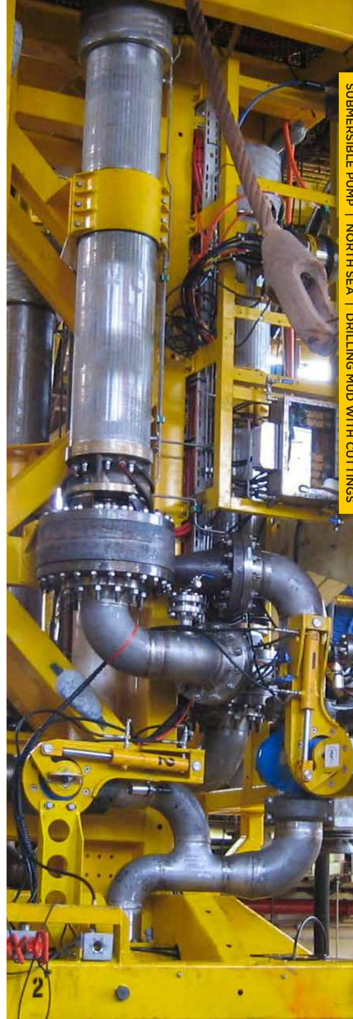
SUBMERSIBLE PUMP | NORTH SEA | DRILLING MUD WITH CUTTINGS
