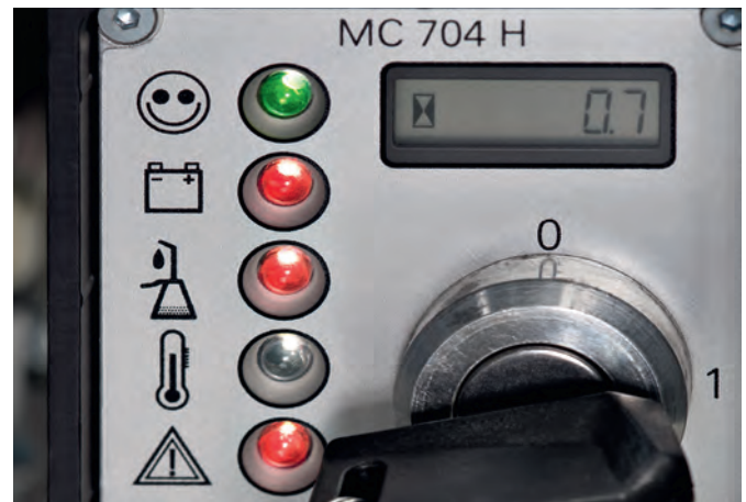
Simple and safe operation: intuitive control, manual pressure adjustment, safety valves and emergency shutdown switch
