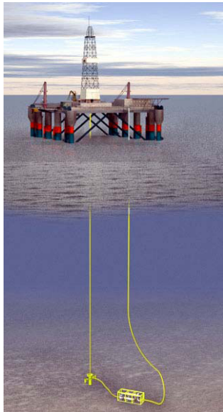
Riserless Mud Pumping System Photo courtesy of AGR Services, Norway
